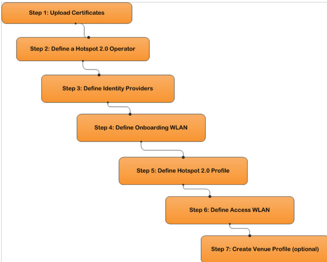
FIGURE 3 Hotspot 2.0 Configuration Flow
